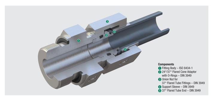
STAUFF Connect 37° Flared Tube Fittings have been developed and designed for the reliable, leak-free connection of tubes with a 37° flare with conventional fitting bodies with a 24° cone according to ISO 8434-1.
